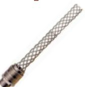
HI-IMPACT **KELLEMS**® Strain Relief Grips are designed to prevent tension from being transmitted to joints and terminals on electrical cord, cable and conduit. In most applications, a grip for strain relief is stronger than the cable/conduit itself, giving greater security than the use of a standard fitting alone.
