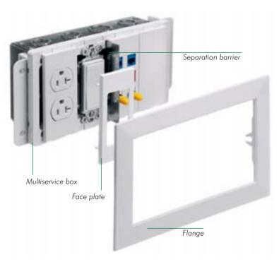
Hubbell MULTI-CONNECT® Boxes provide a versatile "in the wall" solution for single and multi-service applications. Available in 1-, 2-, 3-, 4- and 6-gang boxes, barriers for separation and power and low voltage services, along with a wide variety of modular face plates and wall flanges to match office decor.
