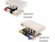
Ideal for open office MUTOA cabling, compact surface mount environments, and retrofits to support data, voice, and multimedia applications. Features adjustable furniture latches to provide an additional mounting option to common ANSI/TIA/EIA standard furniture openings, and solutions requiring fiber. Box bases feature fiber storage posts that can store 1 meter fiber cable after termination.
